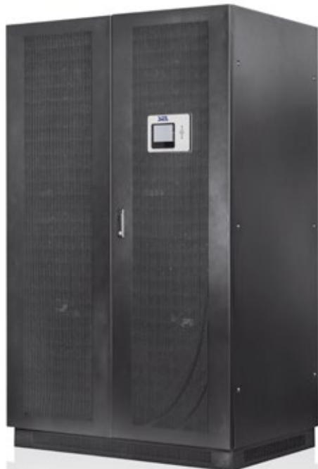
Safepower Modular SPM is based on modular architecture. Each 10-40 kVA UPS module is housed in a single 19" plug-and-play drawer with hot-swap capability. It is virtually a complete UPS. Single points of failure are thus eliminated (de-centralised architecture). In the event a module needs to be replaced, it can be hot-swapped without affecting the operation of the other active modules.
